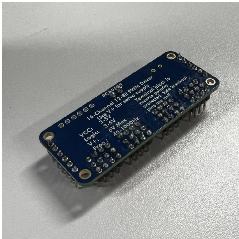
Figure 5 Fully soldered Adafruit
